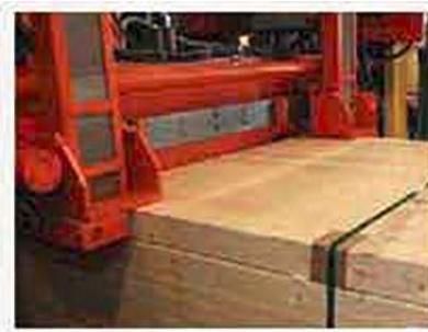
Automatic top and bottom edge protection using flat fibreboard protectors
